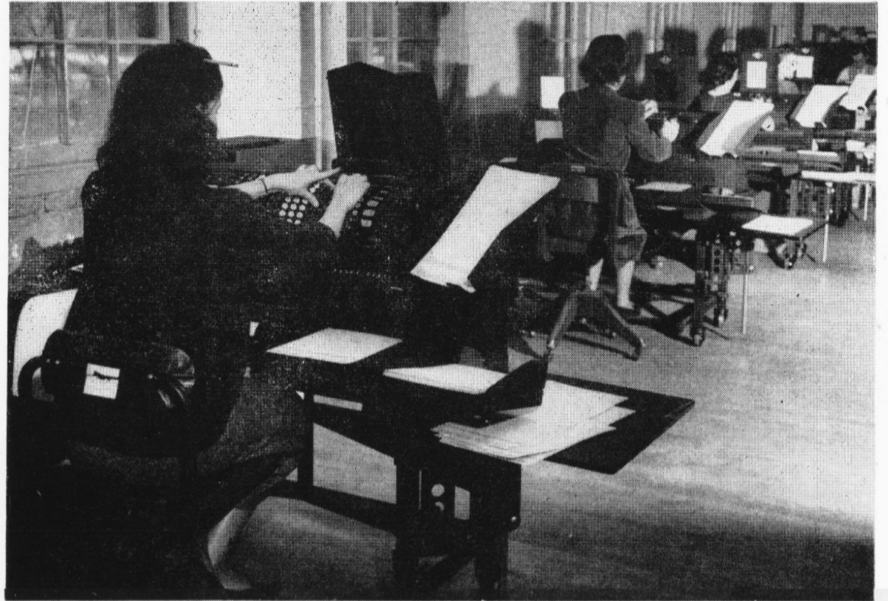
Scovill employees' Wage Statements have taken on a new look since the first of the year. Here are four of the five new Payroll Posting Machines, recently set up in the Central Time Office, that print the Wage Statements. At the same time, they record all the information on other Company records and accumulate totals. That's Shirley Rice at the machine in the foreground.
