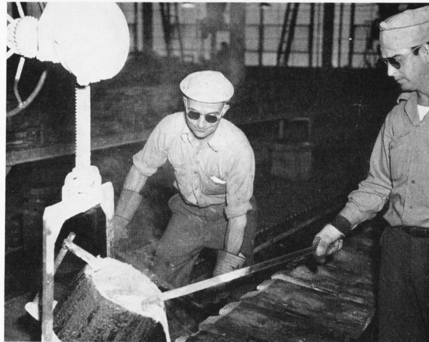
Back at his work in the Waterville Foundry after spending a happy holiday is Frank Ruby (left, above). Frank will tell you it was an especially happy holiday when he thinks of the accident at the Foundry just before Christmas which could have caused him to suffer serious painful burns. That's Bob Whiteway (at right) skimming the molten metal in the crucible.
